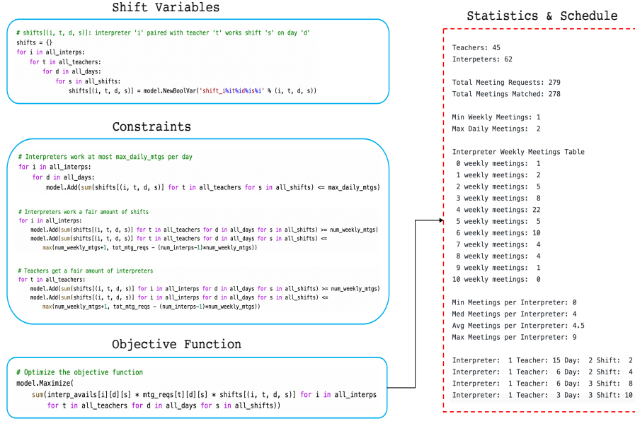
Figure 4. An implementation example of the variables, constraints and objective function the CP-SAT solver utilizes to create a schedule, matching volunteer interpreters with student-teacher conferences. The final output provides various high-level statistics to help describe the final schedule.
